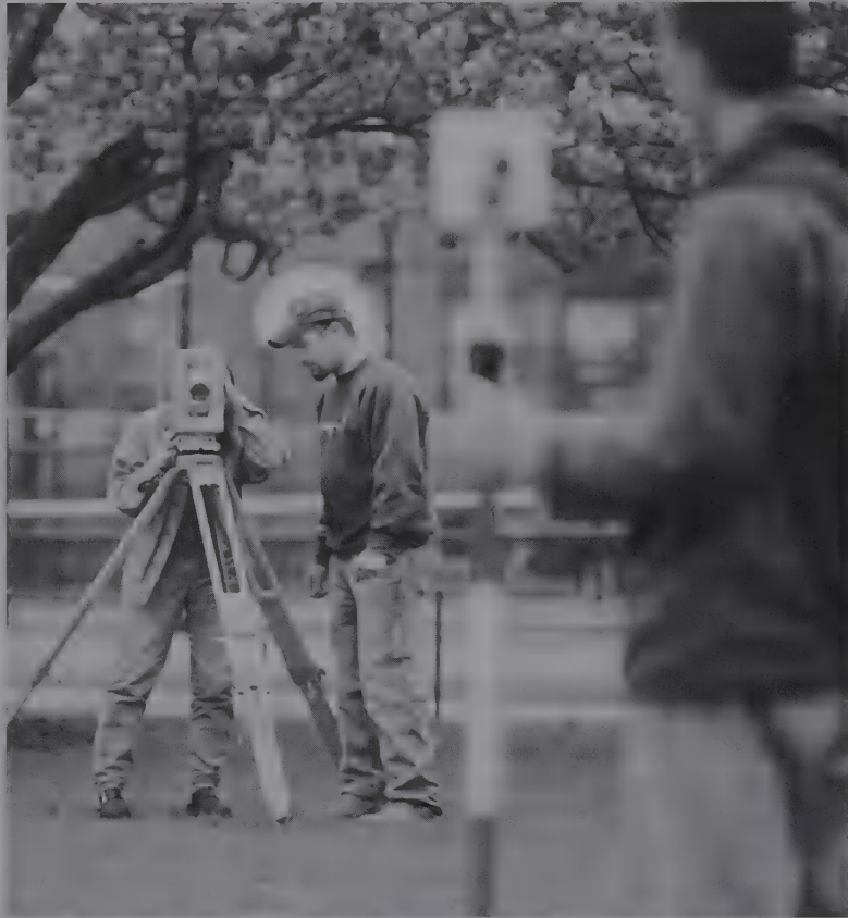
FIGURE 1.2 The total station allows surveyors to collect, record, and transcribe surveying information with greater speed and accuracy
