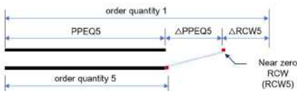
Figure 2. The five scenarios concerning the rebar usage and cutting waste concept.
