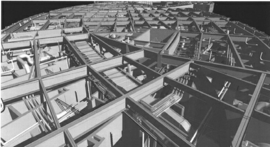
Figure 5.2 Building information model of mechanical work
